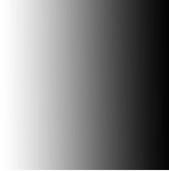
Figure 5.11: Gradient mask used in contrast non-uniformities test.
