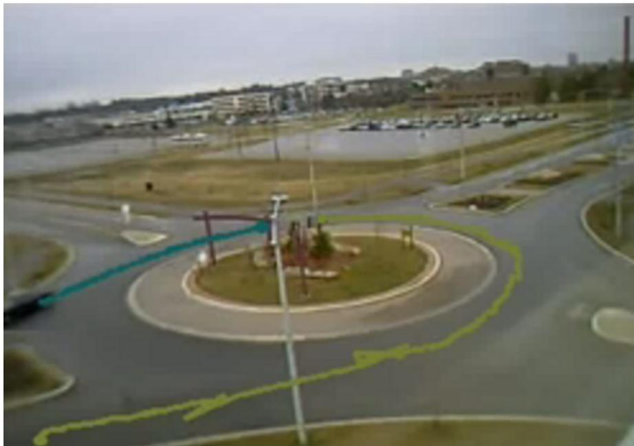
Figure 4.9: Track Split Errors: This figure illustrates an example of a type of tracking error that causes a vehicle to not be counted.
