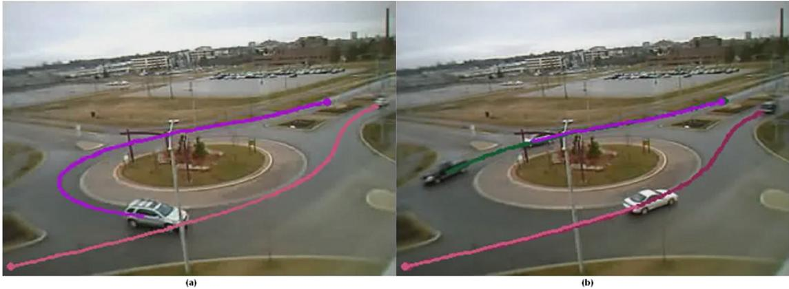
Figure 4.7: Real World Tracking Results: Figure shows tracking results of a roundabout. Each colored track represents a different vehicle.
