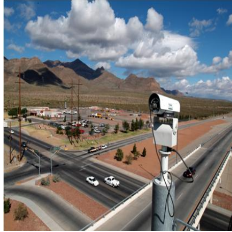
Figure 6.1: Example of a camera mounted on a pole above highways and recording video sequences (Source: Texas Transportation Institute).
