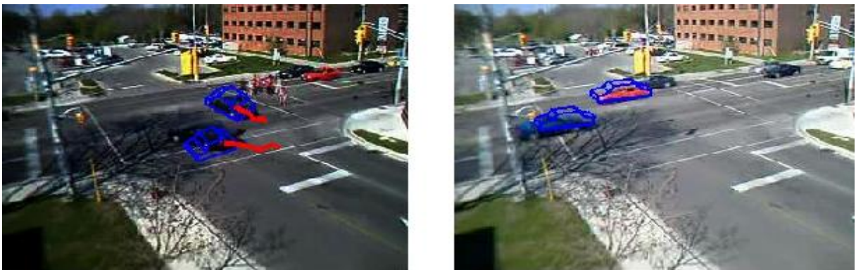
Figure 6.9: The left image is an instance of a video sequence where the grade would be 2. The vehicles that are visible were well detected individually, however the size detected did not cover the whole vehicle (grade 2). The vehicles were recognized and a model was overlapped, but one of the vehicles was given a wrong model orientation (grade 1). The tracking is correct, yet slightly jagged (grade 3). However, the model corrects itself in later frames. The right image is a failure case due to the undetected car behind the red vehicle and the incorrect overlap of the model for the front most car.
