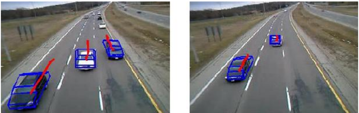
Figure 6.8: The left image is a case where the grade would be 4. The vehicles that are visible were well detected individually and recognized with the model well encapsulating them. Furthermore, the tracking has been correct. The right image is an example of a case when the grade would be 3. Both vehicles are well tracked (grade 4 for module 3) but the segmentation module gets 3 because the size of the model is not covering the whole vehicle and recognition model gets a grade 3 because the model overlap is slightly moved sideways.
