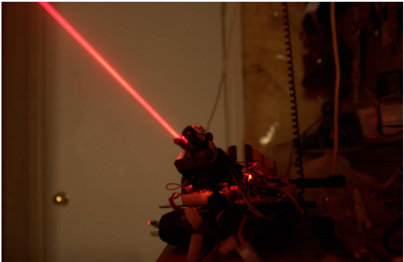
Bottom: Unit with ranging laser activated (steam used to make laser visible)
