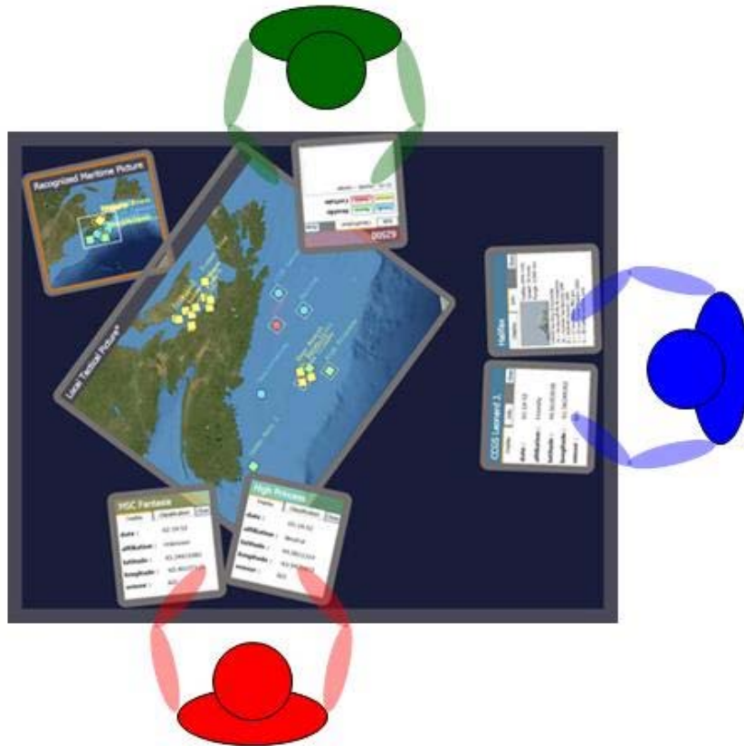
Figure 2. The system provides adjustable windows to enable use from any side of the table.
