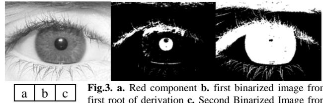
Fig.3. a. Red component b. first binarized image from first root of derivation c. Second Binarized Image from global thresholding
