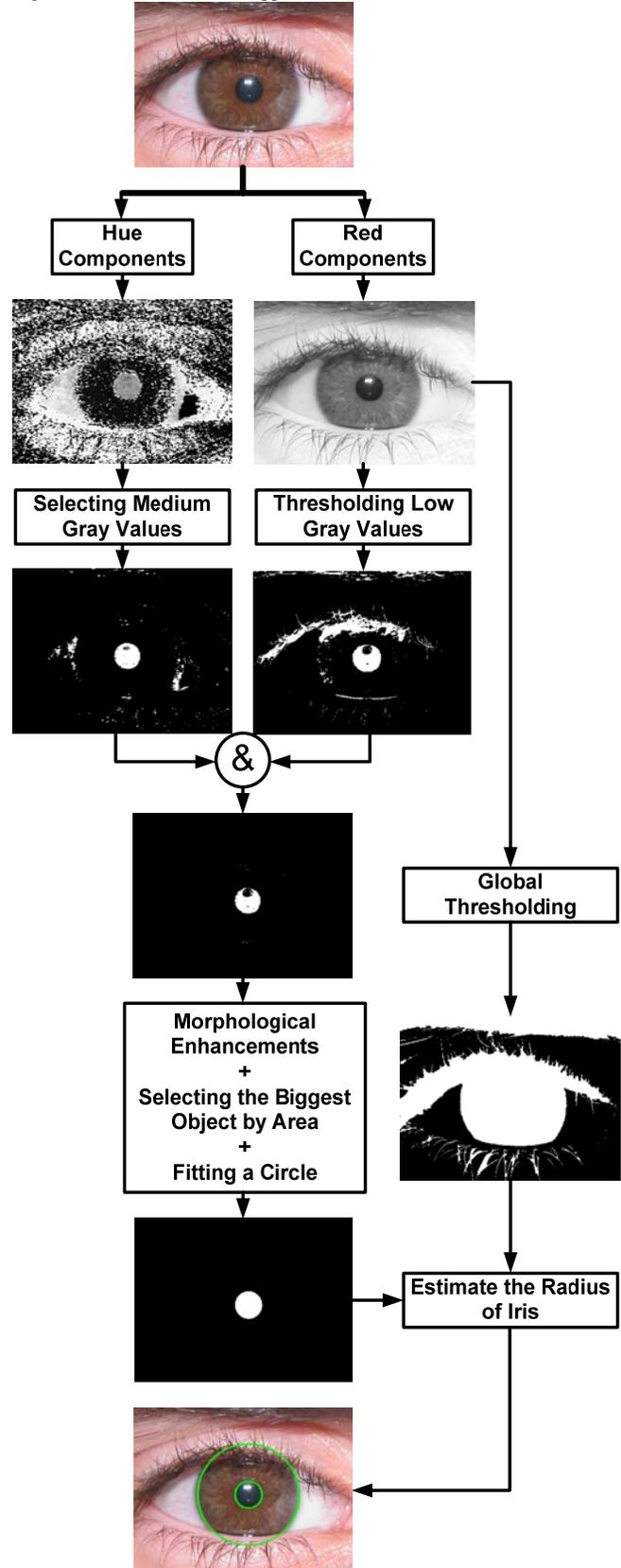
Fig.6. Block diagram of the implemented methodology. The whole procedure of the implemented methodology is shown in figure.6. As it is shown, two binarized image, which
