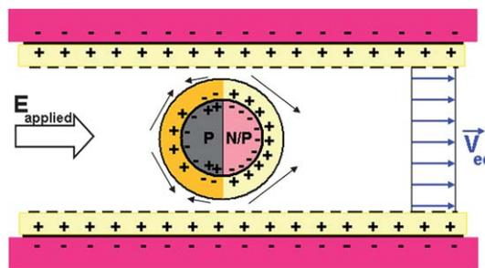
**Fig. 2** The electro-osmotic flow around a Janus particle in a straight microchannel. The arrows represent the direction of electro-osmotic velocity of the flow on different sections of the particle surface.
