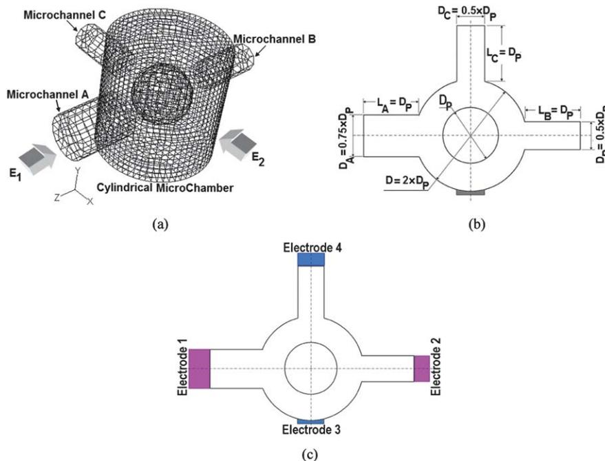
**Fig. 3** Schematic diagram of the micro-valve with three microchannels and one suspended Janus particle in it. (a) Computational domain.  $E_1$  and  $E_2$  represent the external electric field directions. (b) Geometry and dimensions in non-dimensional format. (c) The location of electrodes.
