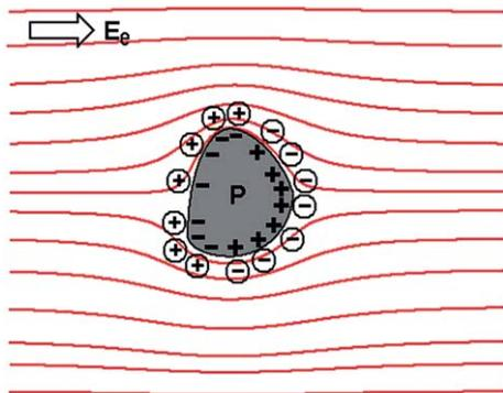
**Fig. 1** Steady-state electric field and the induced dipolar electric double layer around a fully conducting object in an aqueous solution.
